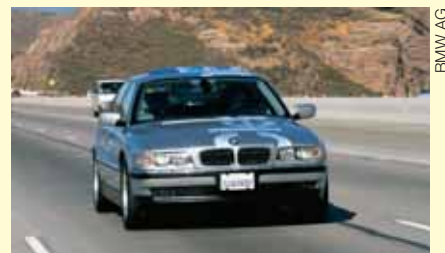
BMW 750hL, hydrogen combustion
